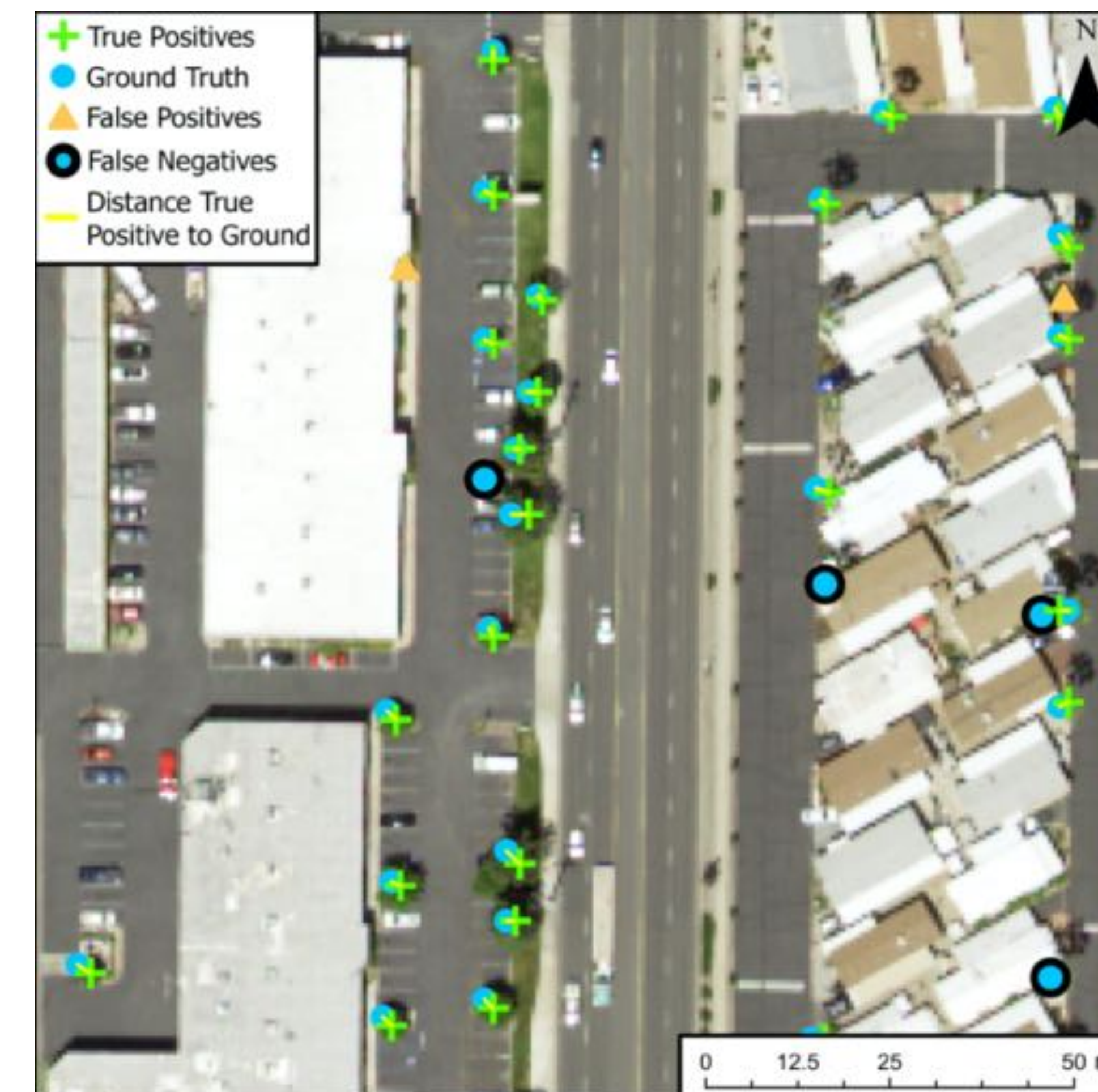
Results from our test data in Claremont, CA. This is an area where the neural network counted trees with high accuracy. Green crosses indicate true positives, blue circles indicate our training data, blue circles with a dark outline indicate false negatives, and orange triangles indicate false positives. We lose accuracy when trees are very dense, shrubs are very large, or there are many shadows in the imagery.
